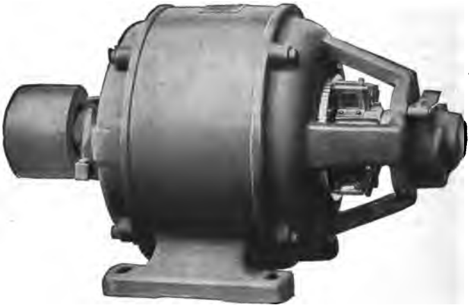
FIG. 275. A single-phase induction motor with commutator and brushes for starting as a repulsion motor. The Westinghouse Electric and Mfg. Co.
